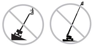
Do not raise or extend the boom unless both axles are extended.
