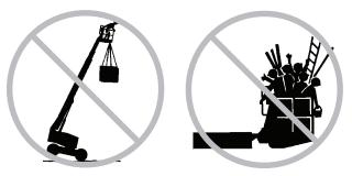
Do not use machine on a moving or mobile surface or vehicle.
